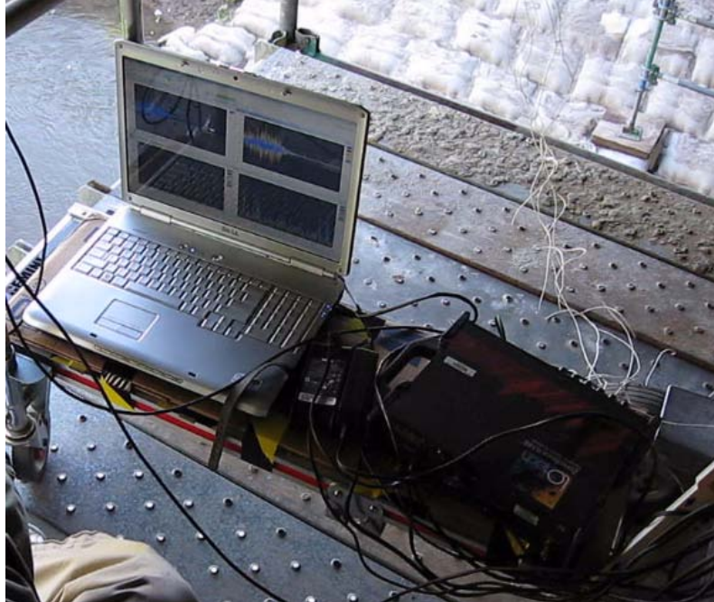
Figure 4.3 Typical field operational vibration test setup
