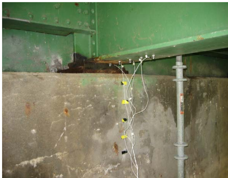
Figure 4.25 Operational vibration response measurement of a beam near the boundary condition
