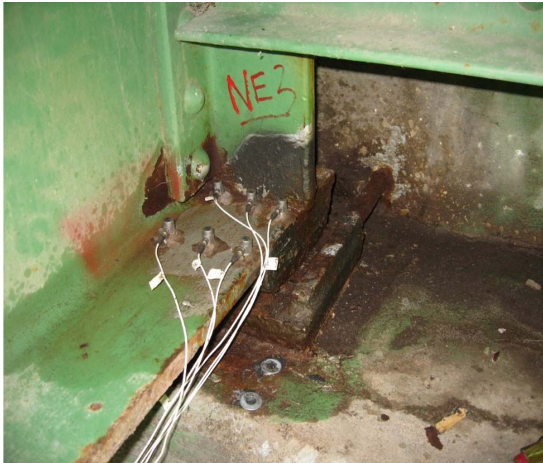
Figure 4.47 Forced vibration response measurement of northeast end and boundary condition of beam 3
