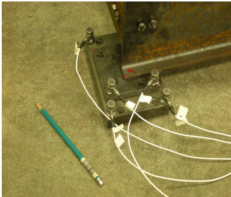
Figure 3.23 Accelerometers fixed with magnets to the first six response points of the scale bridge
