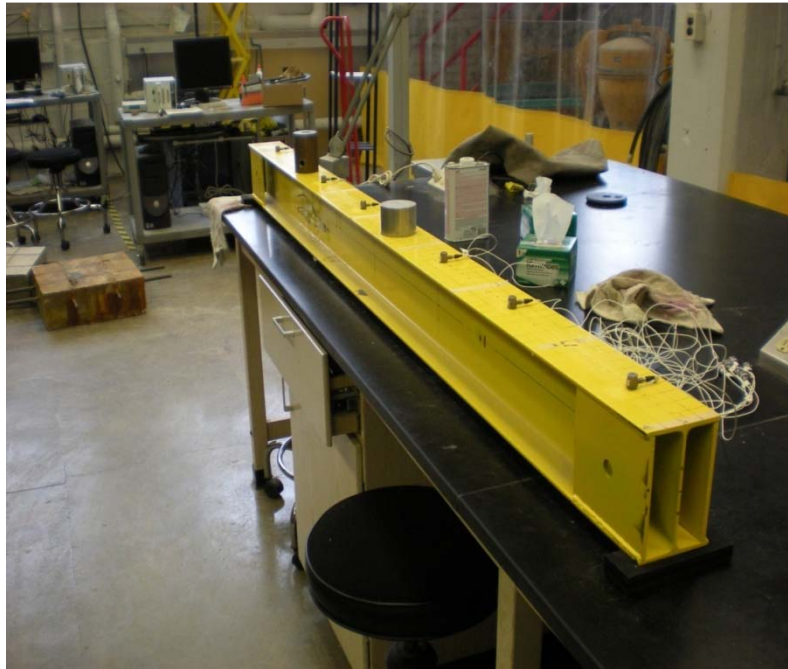
Figure 3.3 Typical laboratory I-beam setup with six fixed accelerometers and two damage zones simulated by fixing masses to the top flange of the structure
